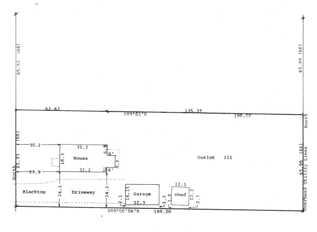
Scale - 1" = 20" $\emptyset = 3/4$ " Iron Pipe Found X = \sqrt{x} X 24" Iron Pipe Set o = 1" X 24" Iron Pipe Set (0.00) = recorded distance Bearings referenced to the assumed bearing of North along the east line of Wood Street Survey ordered by: Churchill Real Estate 322 Park Street Walworth, WI 53184 Updating and recertification ordered by: Churchill Real Estate 322 Park Street Walworth, WI 53184
